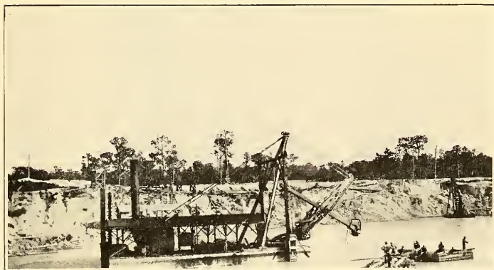
FIG. 4. — MINING PHOSPHATE ROCK BY MEANS OF FLOATING DREDGE.
